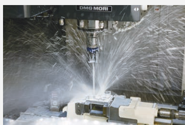
First: High-pressure washing with center through
