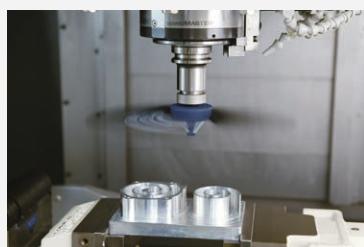
Next: Cleans workpieces and jigs with high Air flow.
